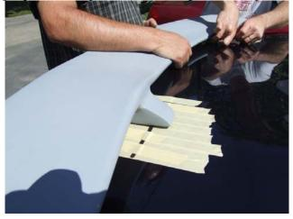
26900 Jefferson Avenue, Murrieta California 92562 951.894.7883, FAX: 951.894.7920 www.rksport.com **4.** Remove the spoiler, leaving the T-straps taped to the vehicle. You will need a 1/8th" bit to drill through the TOP portion where the "pilot holes" are located.
