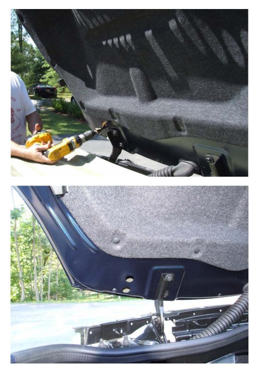
7. Using the <sup>1</sup>/<sub>4</sub>"X <sup>3</sup>/<sub>4</sub>" Pan Head Screws and the <sup>1</sup>/<sub>4</sub>"X1"inch washers, attach the spoiler.
