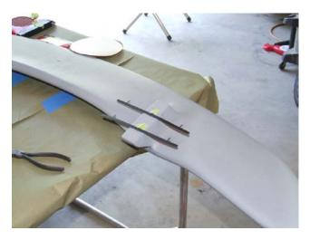
**2**. Place the spoiler on the trunk lid. Line and adjust appropriately ensuring an initial proper fit. Remove the spoiler leaving the "T-Straps".
