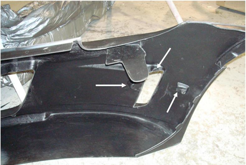
\*\*\* The three arrows point to where the three mounting tabs are for the turn signal assembly. Simply maneuver the assembly to where it lines up with all three mounting tabs and tap the assembly with tapping screws into each mounting tab to secure it into the bumper. \*\*\*
